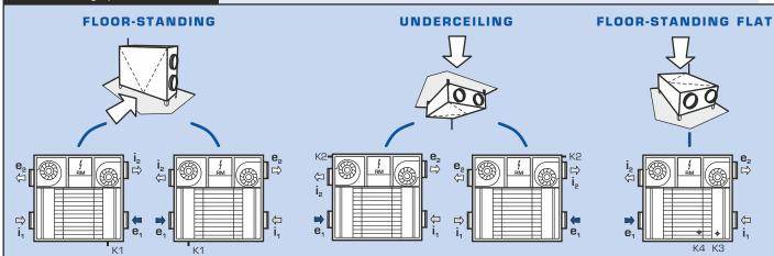
Note: DUPLEX Easy units are supplied for versatile position mounting – the unit can be installed in all positions (floor-standing, underceiling and floor-standing flat). The "right hand" and "left hand" position according to the figure above is selected simply by relocating the operating sensor and by reconnecting unit fans.
